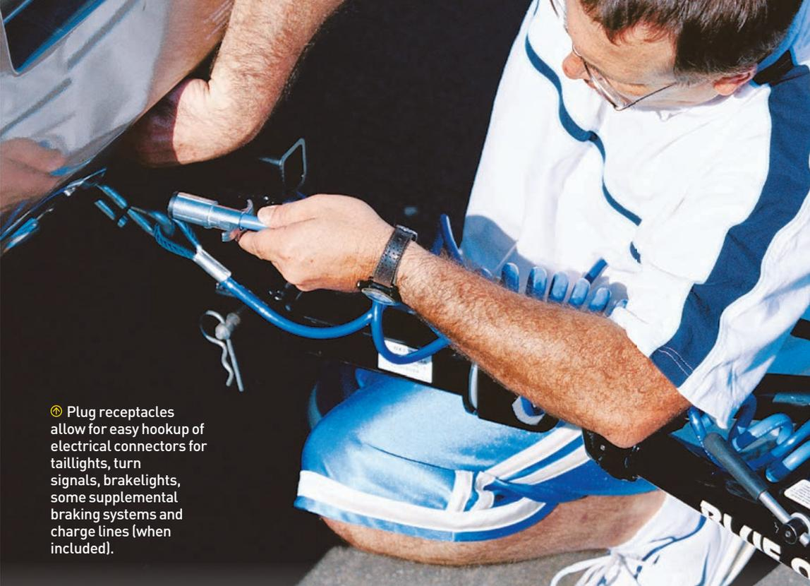
Ⓜ Plug receptacles allow for easy hookup of electrical connectors for taillights, turn signals, brakelights, some supplemental braking systems and charge lines (when included).
